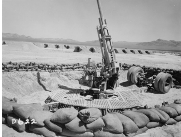
90 mm AA gun, M1A1, at 1500 feet from GZ, project 3.21, 5 May 1953.
